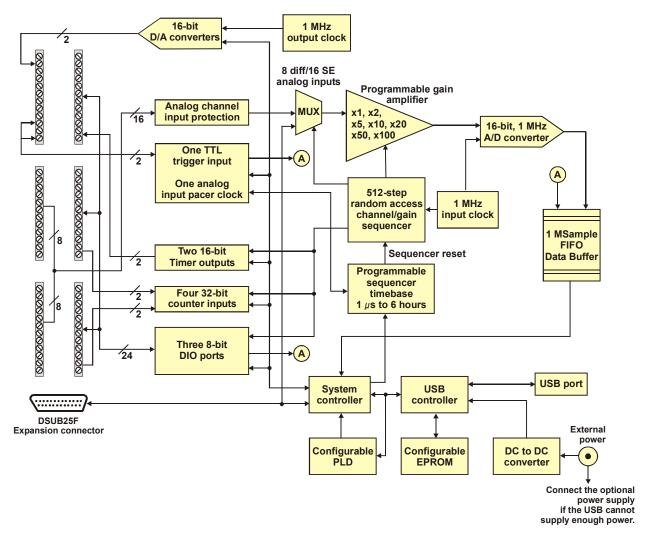
Figure 6. USB-1616HS-2 functional block diagram
